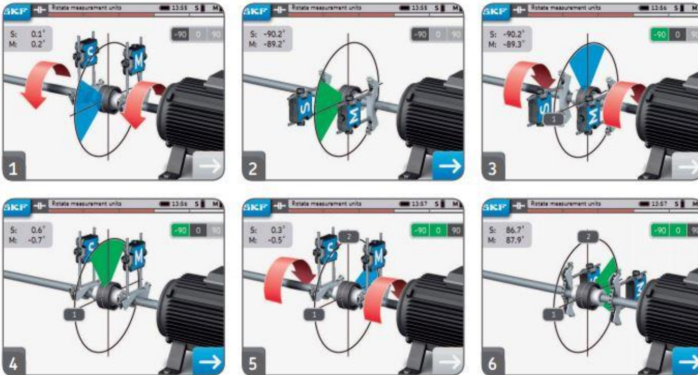
Fig. 5. SKF Shaft Alignment Tool TKSA 31
